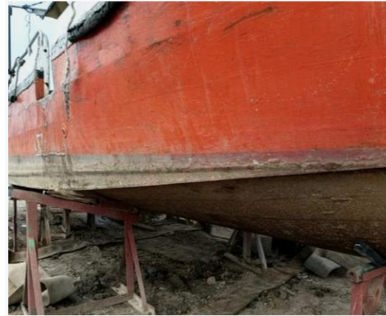
BEFORE / WORN COATING
